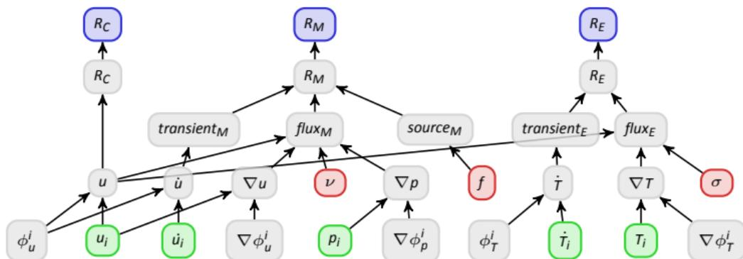
$$R_M = \int_{\Omega} \left( \frac{\partial u}{\partial t} + u \cdot \nabla u - \nabla \cdot (\nu \nabla u) + \nabla p - f \right) \cdot v \, d\Omega, \quad R_C = \int_{\Omega} (\nabla \cdot u) \cdot v \, d\Omega, \quad R_E = \int_{\Omega} \left( \frac{\partial T}{\partial t} + u \cdot \nabla T - \nabla \cdot (\sigma \nabla T) \right) \cdot v \, d\Omega$$
