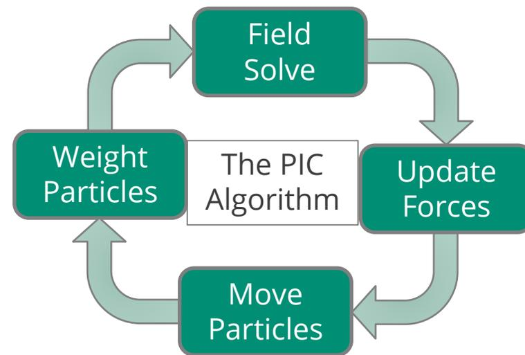
Flow diagram showing a pure PIC timestep<sup>1</sup>
