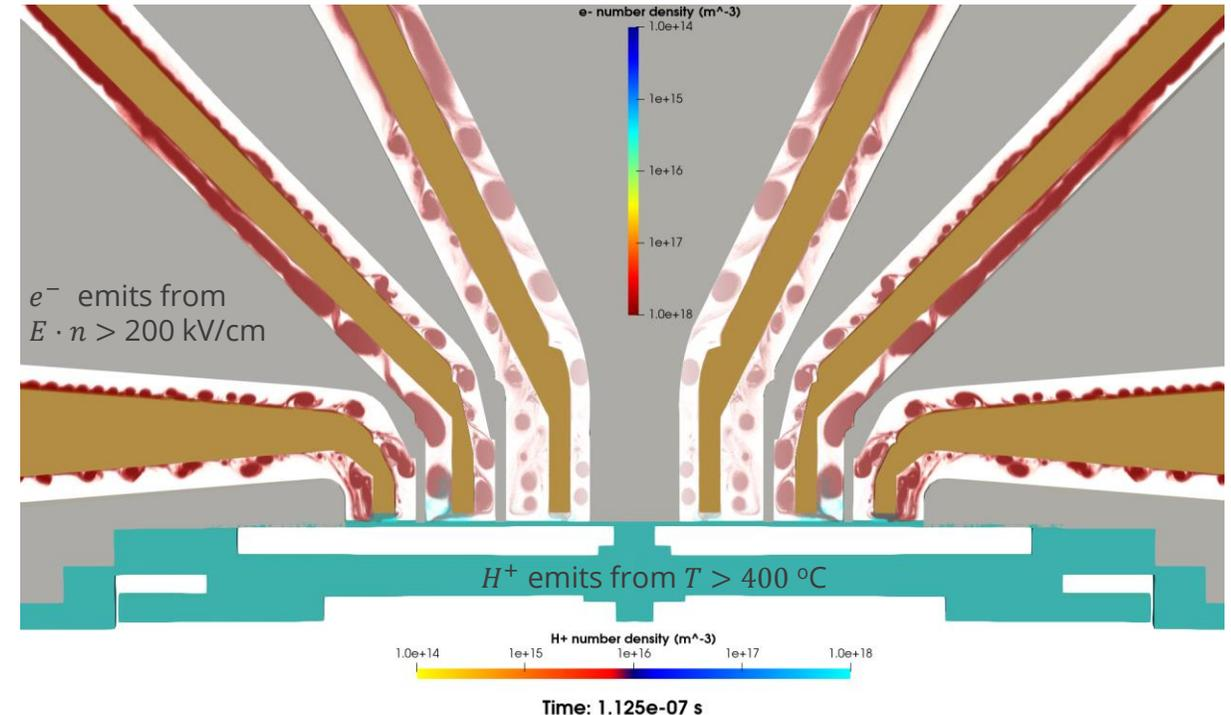
**spatially- and time-resolved simulation of bipolar flow**
