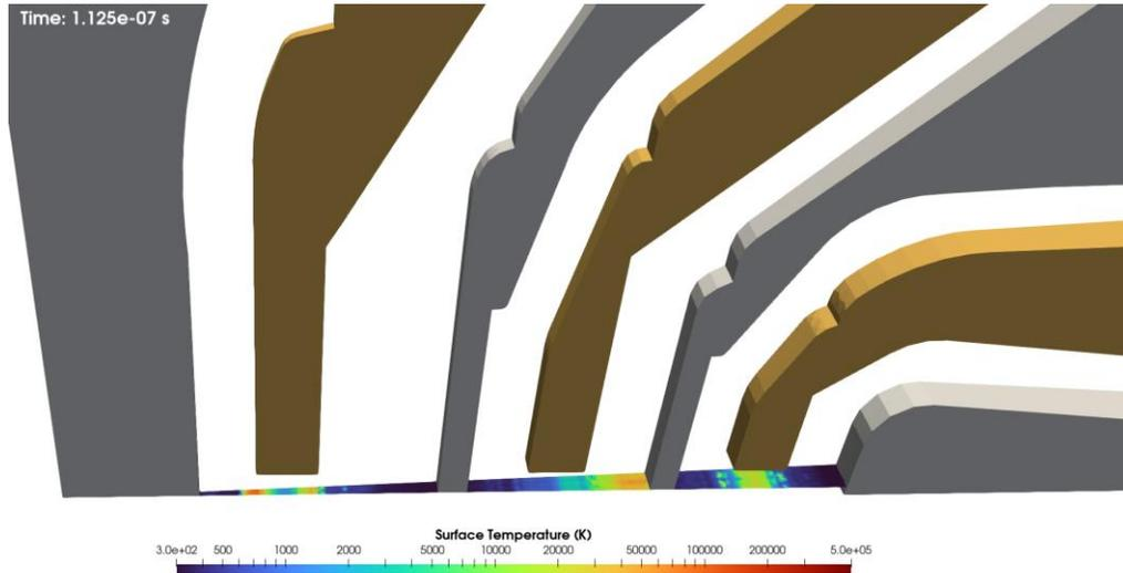
We simulate  $2.5^\circ$  azimuthally-periodic domains using 28-87M element meshes on 90-350 HPC nodes. Each simulation takes  $\approx 20$ -30 wall-hours
