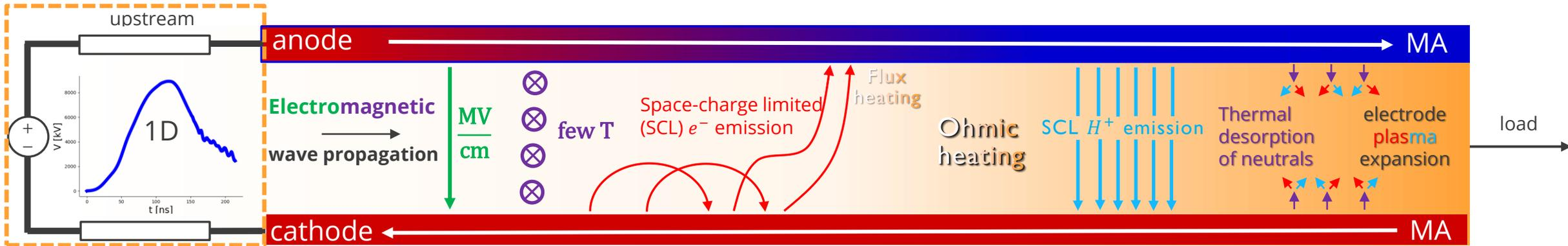
**Solution:** 1D-3D computational model – TEM wave propagation in 1D transmission line domains (meters) are coupled to a single 3D EM-PIC domain downstream (centimeters) simulating the details MITL physics
