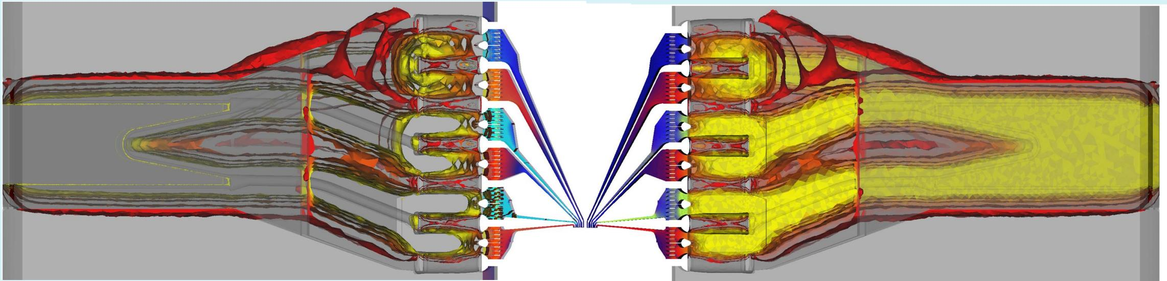
Open contours of electric field magnitude show areas of high field gradient while tri-plate structure is recognizable
