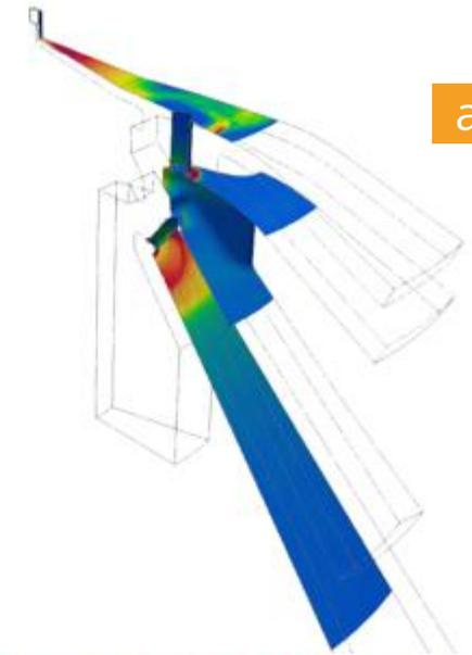
anode heating from  $e^-$  fluxes
