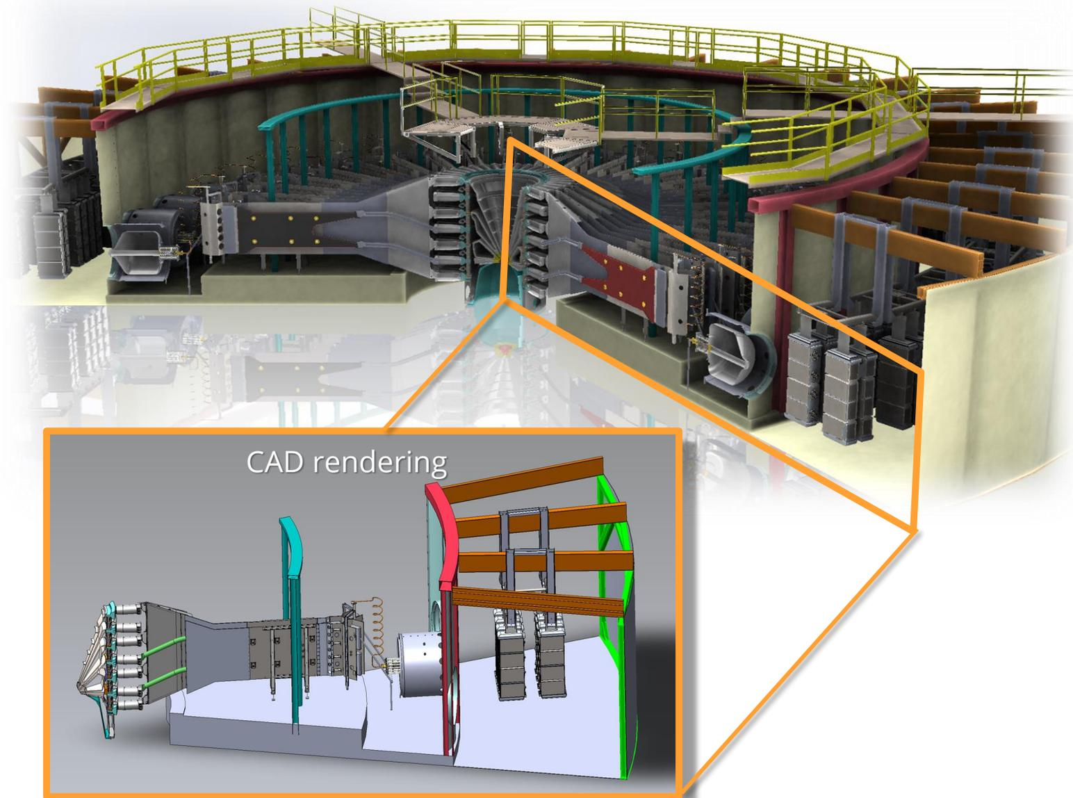
A large-domain 3D electromagnetic model was developed to characterize power flow from the Saturn **water line** to the load
