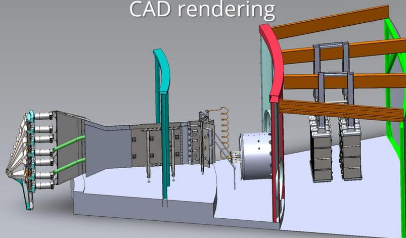
A large-domain 3D electromagnetic model was developed to characterize power flow from the Saturn **water line** to the load
