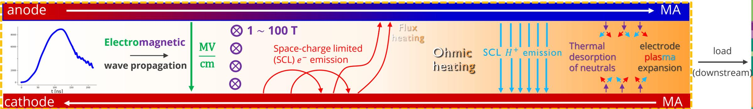
Most germane processes to correctly simulating pulsed power operation, i.e. a non-exhaustive list!
